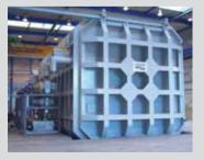
Electron-beam welding can be performed in large vacuum chambers whose volume is comparable to that of a singlefamily home.
